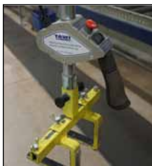
Fork tool used for lifting large aluminum profiles
