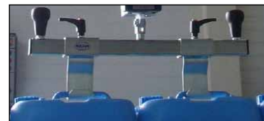
lifting two containers at a time with a mechanical tool. Two adjustable hooks on a yoke.
