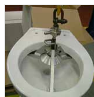
Two different types of clamping tools used with to lift ceramic toilet seats.
