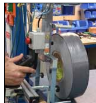
Roll handling pneumatic gripper, paper roll with adjustable joystick control
